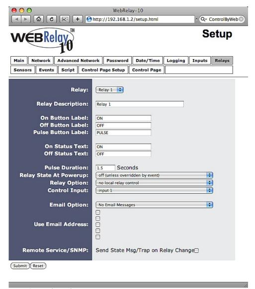
Figure 2.4i - Relays Tab
