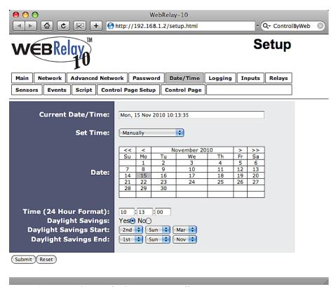
Figure 2.4e - Date/Time Tab - Set Time Manually
