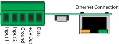
Figure 2.2c - Connector Pinout
