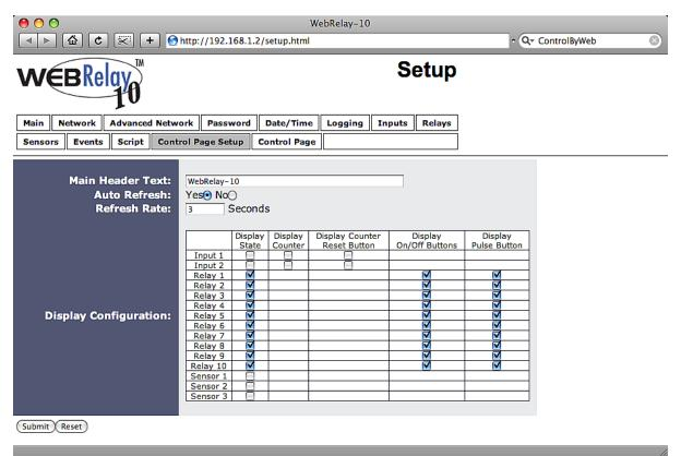
Figure 2.4p - Control Page Setup Tab
