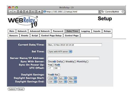
Figure 2.4f - Date/Time Tab - Sync with NTP Server
