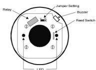
Fig. 4 Schematic of detector Structure When front cover is open.
