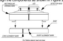
Fig. 2 Mating detector head onto base
