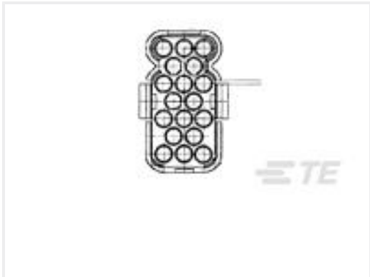
TE Part #925450-1 M-N-L PIN HSG
