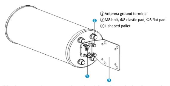
(2) Tighten 2xM8 U-shaped screws with 2xU-shaped clamp plates and L-shaped support plates with 4xM8 nuts,  $4x\Phi8$  elastic pads and  $4x\Phi8$  flat pads, and pay attention to the antennas to be perpendicular to the ground.
