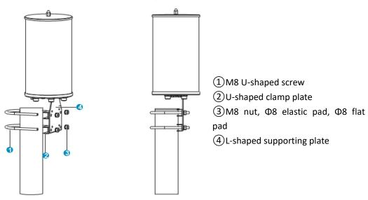
(3) After the installation is completed, the grounding cable needs to be connected, please ensure that the grounding terminal is reliably grounded.
