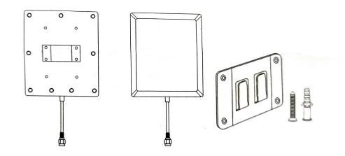
Step1 : Take the material out of the bag and fix the flat plate against the wall with the four screws.
