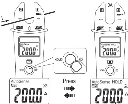
Data Hold is not available when "OL KΩ" displayed with no input signals.
