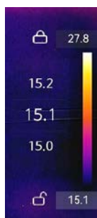
Figure 3-10 Level Only Adjustment
