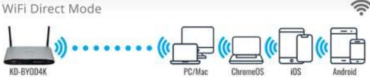
**WiFi Direct Mode** allows wireless devices direct access to the base unit. Any additional wireless devices on the local network can access the base unit via LAN if it is connected to a wired local network.
