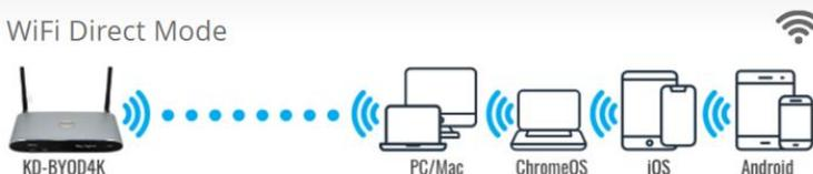
**WiFi Direct Mode** allows wireless devices direct access to the base unit. Any additional wireless devices on the local network can access the base unit via LAN if it is connected to a wired local network.
