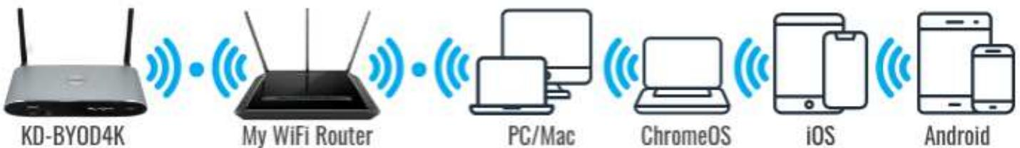
**LAN Connect Mode** requires KD-BYOD4K be wired into your local network. Wireless devices access KD-BYOD4K via your existing external WiFi network therefore allowing users to stay connected to an internet enabled network(s). WiFi Direct mode is disabled when LAN Connect Mode is enabled.
