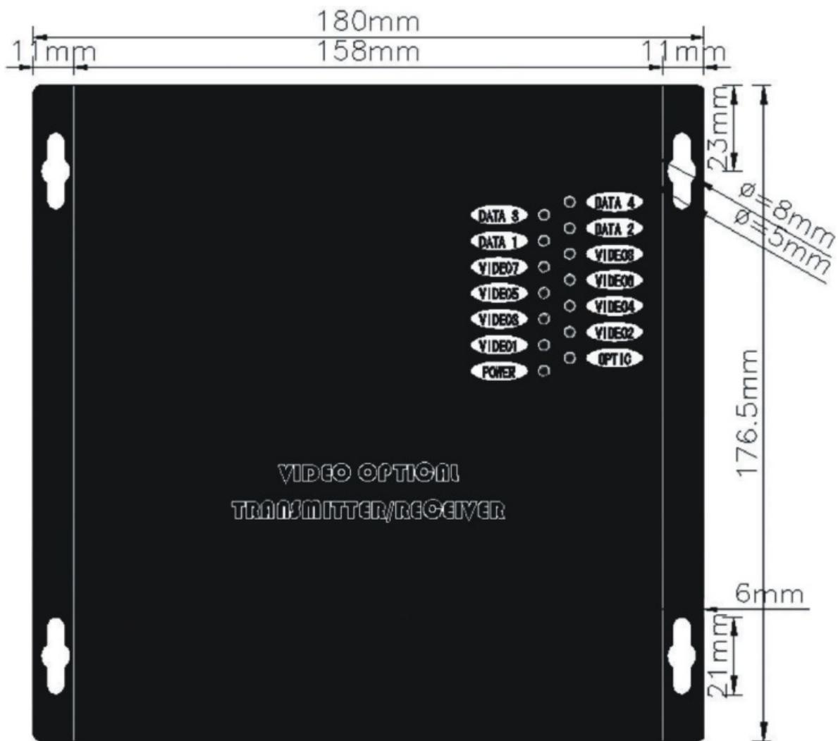
The 20100077 transmitter/ receiver can be installed into our rack mount chassis, TBD, which can be mounted into an industry-standard 19-inch equipment rack.
