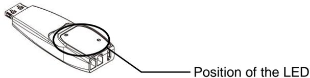
Figure 2 – Position of the LED
