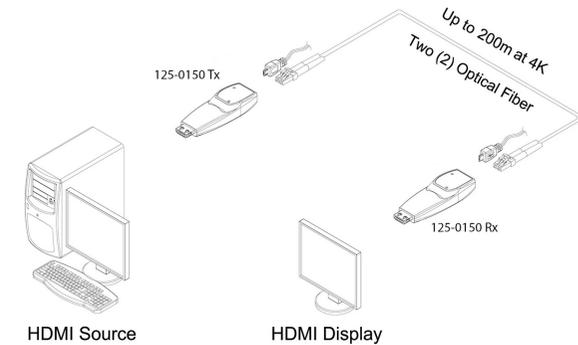
Fig Figure 4 – Connection with optical fiber
