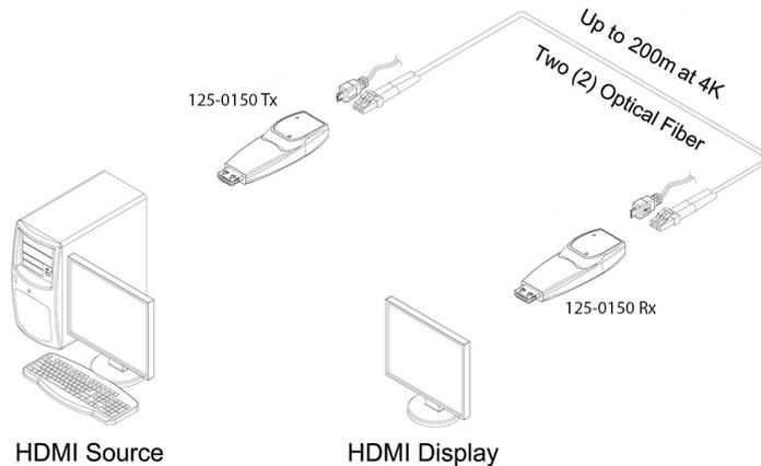
Figure 1 – Overall Connection of 125-0150
