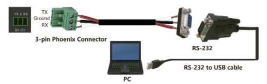
Next, open a Serial Command tool on the PC to send ASCII commands to control the device. The ASCII command list is shown below:
