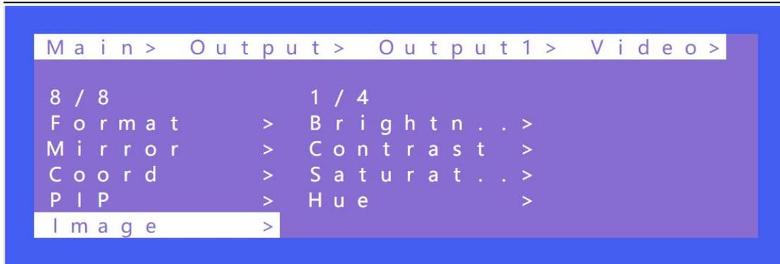
Picture- set the parameter of the output image
