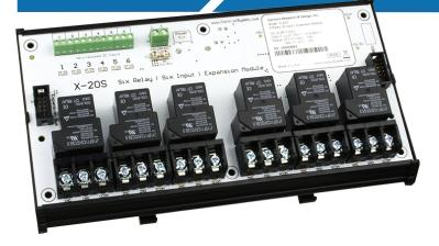
The X-20s™ expansion module is used with the X-600M controller. The X-20s has six, high-current relays, each with Form-C contacts (SPDT) and six, optically-isolated digital inputs. A screw terminal strip provides high-current connections to the relays.
