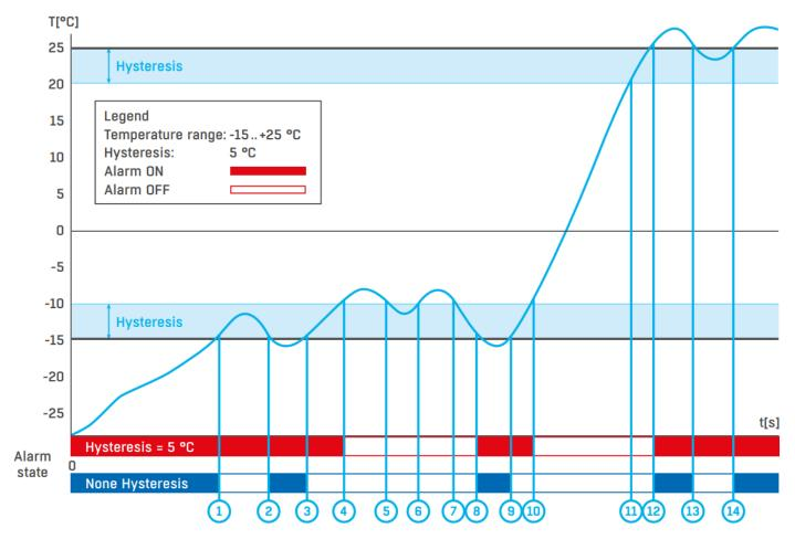
Within the internal 5°C hysteresis band, the alarm would be activated at **point 8** and would end at **point 9**. Because of the hysteresis function, the alarm is extended until the temperature reaches the end of the hysteresis zone (point 10) 5 °C + (-15 °C) = -10 °C.
