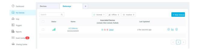
2. Go to "My Devices" page and click "+New Devices". Fill in the SN of the device and select an associated gateway.
