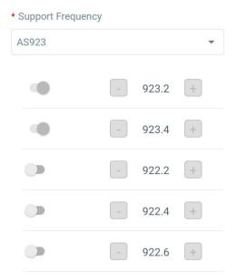
If frequency is one of CN470/AU915/US915, you can enter the index of the channel that you want to enable in the input box, making them separated by commas.
