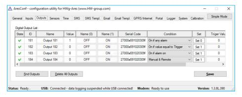
It is possible to connect the External Outputs module via the 1-Wire UNI interface to the Ares 12 LTE device. This module provides 4 NO/NC relay outputs with maximum load up to 1A/30VDC or up to 0.5A/50VAC.
