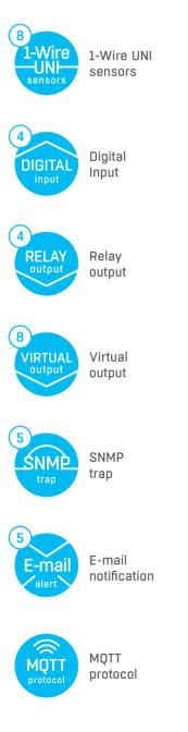
Poseidon2 3268 supports up to 8 sensors connected over 1-Wire UNI / 1-Wire and up to 4 detectors connected to digital inputs. Poseidon2 3268 can control 2 digital NO/NC relay outputs, as well as up to 8 virtual digital outputs (VDO) at remote Poseidon2 or Damocles2 units (M2M).
