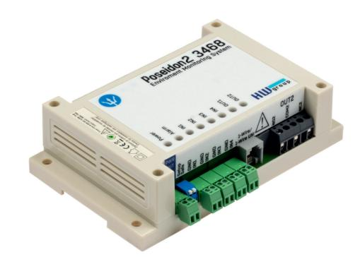
Poseidon2 3468 supports up to 8 sensors connected over 1-Wire UNI / 1-Wire and up to 4 detectors connected to digital inputs. Poseidon2 3468 can control 2 digital 230 V / 16 A relay outputs, as well as up to 8 virtual digital outputs (VDO) at remote Poseidon2 or Damocles2 units (M2M).
