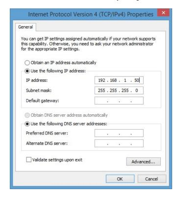
Select the radio button labeled "Use the following IP address" and type in the IP address:
