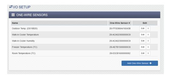
To add a new local one-wire sensor click Add One-Wire Sensor in the local 1-Wire Sensors Table.
