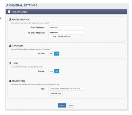
webrelay (all lower case). The password access for *Managers* can be enabled or disabled. When a manager logs into the setup pages, they will receive a subset of the menu options allowing them to edit Scheduled Tasks and view the control pages.
