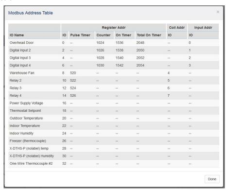
For example, to pulse Relay 3, write a 32-bit floating-point value in the endianness defined starting at register 524 and ending at register 525. Most Modbus programs do this by setting the start address to 524 and writing a quantity of two registers.
