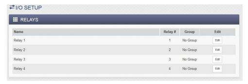
Click the respective edit button to configure each relay. Local relays have some settings that remote relays don't have and vice versa.
