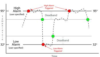
For example, if the Deadband is set to 1 degree, and a high alarm is occurs at 95
