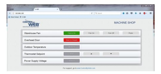
The Control Page is normally what users see and use and it can be highly configured to fit your needs. The Monitor & Control Tab > CONTROL PAGE SETUP tab has settings that determine what resources are displayed and how they are formatted.
