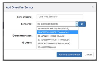
Enter a descriptive name for the sensor in the *Sensor Name* box such as "Outdoor Temperature". The text in this field appears to the left of the corresponding temperature/humidity reading on the Control Page. This text also appears in the email status message when email is enabled. When later defining the control logic, logging and other settings, this label appears in the pull down lists of sensor resources. This field can be up to 27 characters in length.
