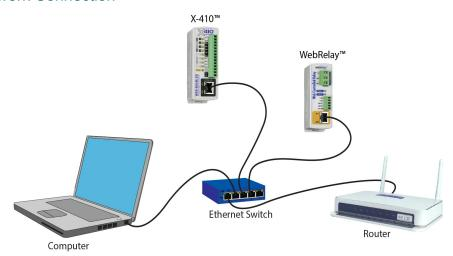
Connect the Ethernet port to a standard 10/100/1000 Base-T Ethernet connection. The X-410 typically connects to an Ethernet switch, or router. For configuration, X-410 may be connected directly to the Ethernet port on a computer or through a switch or router. The X-410 supports auto negotiation and will work with either crossover or straight-thru cables. The X-410 can be used on a wireless network by connecting through an Ethernet bridge or a wireless router.
