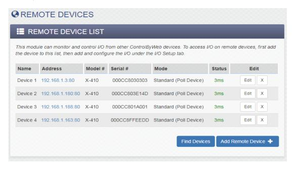
To add a remote device, click *Add Remote Device*. Depending on the *Model* selected in the pull down ▼ list, the available settings will change to accommodate the capability's of the remote device. For example, only certain devices can support encrypted communications.
