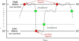
For example, if the Deadband is set to 1 degree, and a high alarm is occurs at 95 degrees, the
