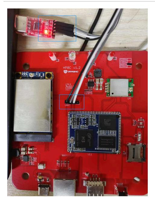
In the PC, you can use the serial port tool(such as <u>putty</u> in Windows), you need to set the serial baud rate to **115200** to access the serial console for LPS8v2. LPS8v2 will output system info once power on as below:
