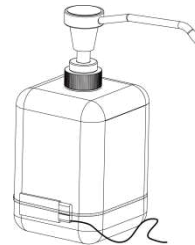
Fixed by Cable-tie
