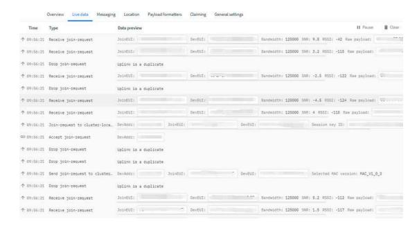
After join successful, LTC2 will send uplink message with the sensor value.
