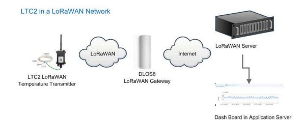
The DLOS8 is already set to connect to <a>TTN</a>. Rest we need to is register the LTC2 to TTN v3:
