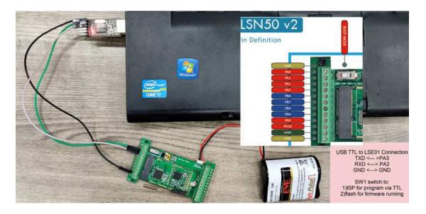
In the PC, you need to set the serial baud rate to **9600** to access the serial console for LSN50. LSN50 will output system info once power on as below:
