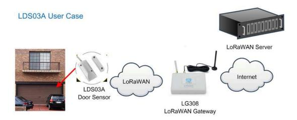
In this user case, the LDS03A is installed on the door edge to detect the open/close event and send the status
