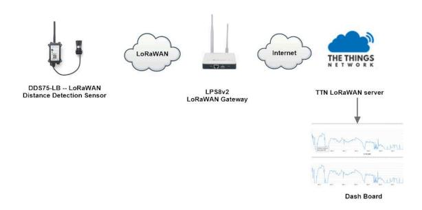
**Step 1:** Create a device in TTN with the OTAA keys from DDS75-LB.
