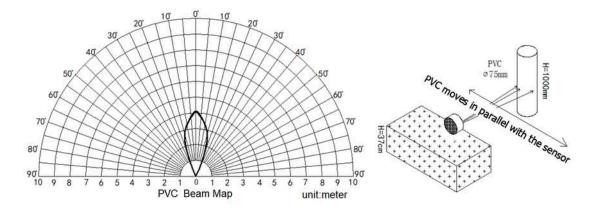
2. The object to be tested is a "corrugated cardboard box" perpendicular to the central axis of 0  $^{\circ}$ , and the length \* width is 60cm \* 50cm.
