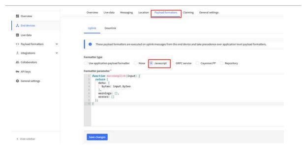
The payload decoder function for TTN V3 is here:
