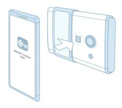
4. Basic information and settings of devices will be shown on ToolBox if it's recognized successfully. You can turn on/off the device by tapping the button on the Device Status. In order to protect the security of devices, password validation is required when configuring via unused phone. Default password is **123456**.
