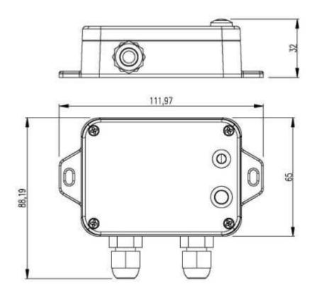
Fig. Main unit housing size
