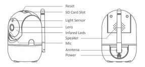
Reset: Long press with the needle for 5s to reset the camera SD Card Slot: Support local SD Card storage (Max 128GB) Light Sensor: To control the IR switch in night Lens: 3.6mm 110degree view lens IR Leds: 6pcs IR leds inside with 10m IR distance Speaker: Support two way audio so you can hear the voice Mic: Capture sound for your video Anntena: 5DB anntena to get wifi access
