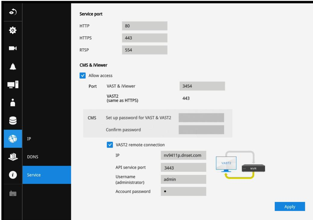
Instead of a web console, you can also access the NVR and the subordinate cameras using the **iViewer** and VIVOTEK's **VSS** software. The NVR can be managed as one of the sub-stations in a hierarchical device structure.
