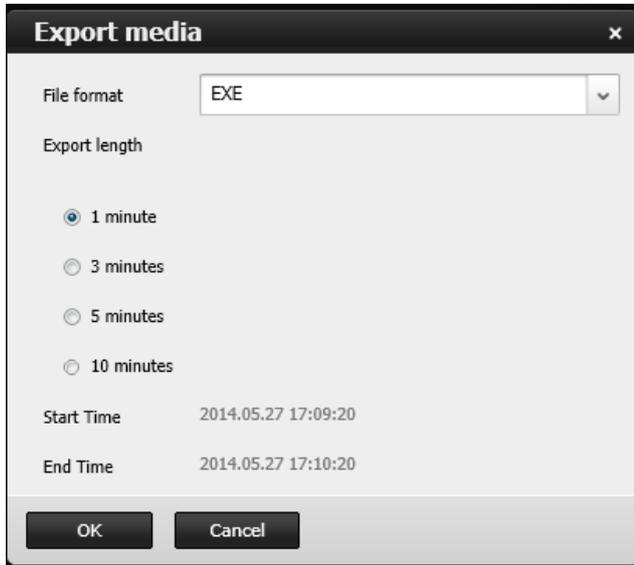
3. Select the file format using the pull-down menu. An **EXE** file is an self-executable file playable by an embedded Media Player. The 3GP format is a multimedia container format for 3G UMTS services. These files can be played on QuickTime, RealPlayer, and VLC. The file name will look like this: [MAC]\_ [DATE]\_[TIME]\_ [CAMERA\_INDEX].[3gp/exe].
