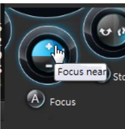
**Auto Focus:** If your camera supports the auto focus function, use this button to acquire an optimal focus point.
