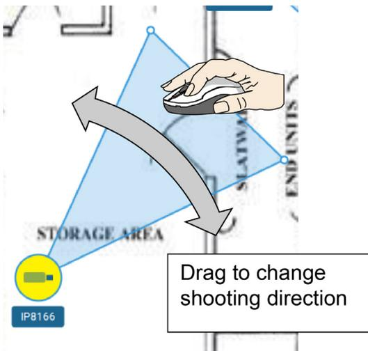
Click on the camera icon. You can also change the color of camera icon and the FOV type. Fisheye cameras, when ceiling mounted, have a round shape coverage.
