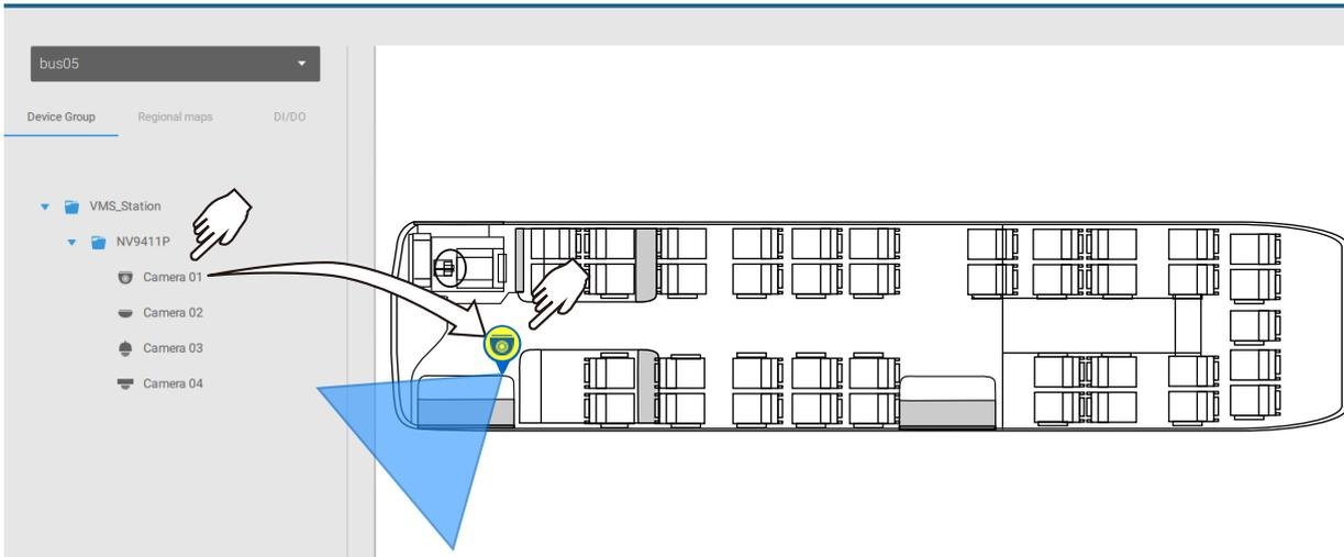
When the camera is in place, drag the FOV indicators on the edge to change the shoot angle and the coverage range.
