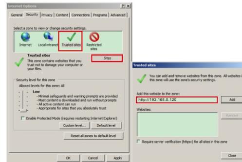
**Step 2** In **Microsoft Edge**, choose **Control panel > Internet Options > Security > Custom level**, and set **Download unsigned ActiveX control** and **initialize and script ActiveX controls not marked as safe for scripting under ActiveX controls and plug-ins** to **Enable**, as shown in figure 4-4.
