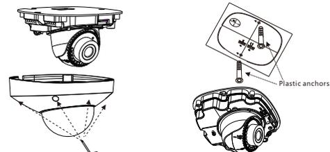
**Step 3** Fetch two black self-tapping screws from the accessory package. Then fix the screws to fasten the camera on the ceiling as shown in figure 3-2.
