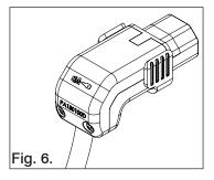
Replace the cord grip (Fig. 4 & 5.) ensuring the torque value is achieved (0.3Nm), and then replace the outer housing and screws (Fig. 6.).
