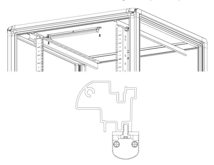
On all other cabinets, fix the light with built in magnetic in any position required.
