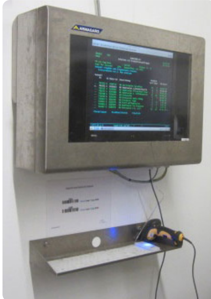
Image: A 24" wall mounted SDS enclosure with optional keyboard tray for Fungers Feinkost, Germany.
