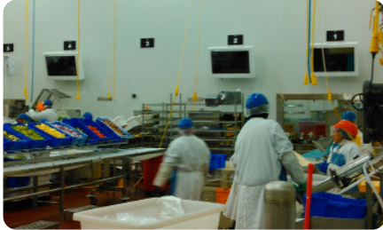
Image: Three 42" wall mounted SDS enclosures, for a Taylor Farms production line, USA.
