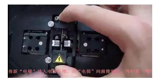
Insert new pair of electrodes and tighten screw.
