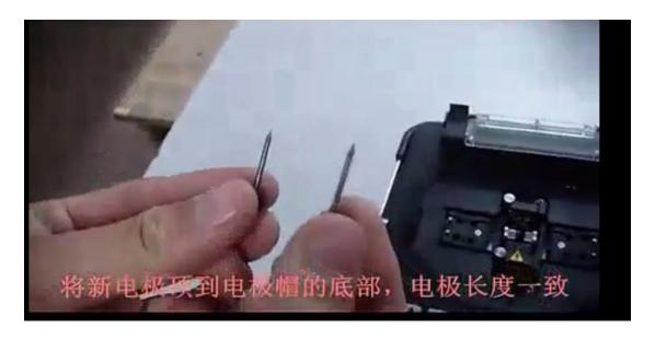
Make the new electrode to the bottom of the electrode cap. Make the two electrode in same length. As the above photo.
