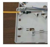
Pic8: right-routing leads in box and fixes by nylon tie
