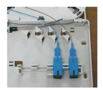
Pic11: install the adaptor and pigtail
