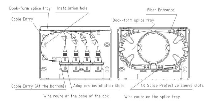
Pic1: The fiber route schematic diagram
