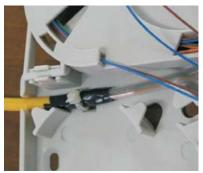
Pic12: put the pigtail through into thePic13: pigtail inserted the tray
