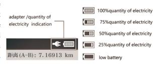
Battery power will be displayed at the top of the screen. When the power is too low, a warning message will appear. Please connect the instrument to the power socket with a random adapter and charge it in time.
