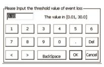
Setting method: Under the parameter setting interface, press [Event Loss Thre.], pop up the event loss
