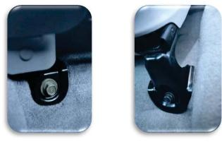
3. Mounting base options: There are several options to set up your mounting base. Please find the setup option that best fits the seat bolt and seat rail design under the front left corner of your passenger seat.
