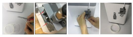
4. Press the Knob to start loading filament. Once filament starts extruding from the Nozzle, press the Knob again to stop extrusion. Clean the extruded filament, then press the Knob to select the Continue option.
