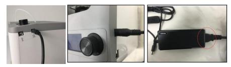
7. Flip the power switch on the inline control to the ON position (I). After the printer finishes booting, you will see the following wizard. Depress the Knob on top of the printer to select Next on the Welcome Screen, then again to select Next on the STEP 1: LOAD FILAMENT Screen.
