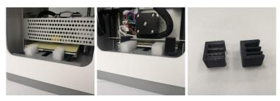
4. Rotate the Coupling Screw clockwise to lift the Magnetic Print Bed, then remove the foam block from under the print bed.
