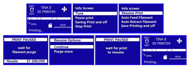
With the Printing... Screen displayed, press the Knob to display the Print Control Menu.
