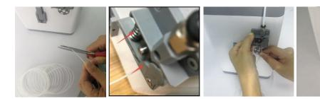
9. Press the Knob to start loading filament. Once filament starts extruding from the Nozzle, press the Knob again to stop extrusion, then press the Knob to select the Continue option.
