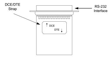
Figure 3. DCE/DTE strap orientation on PC board
