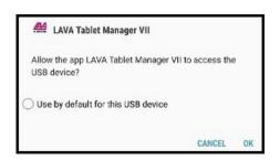
The LAVA Tablet Manager (LTM) suppresses the USB permission pop-up window for peripherals, using the Samsung KNOX SDK.
