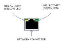
The USB Activity is a yellow indicator. The USB Activity is solid yellow when the LAVASynC+ is powered and connected to the device. The USB Activity flashes when there is traffic between the device and a LAVASynC+ product.
