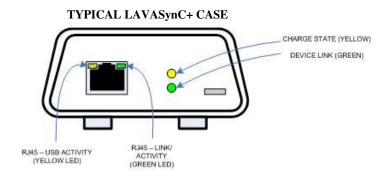
Units with Ethernet support have two additional status LEDs mounted in the RJ45 receptacle, which are described in the ETHERNET RJ45 section.
