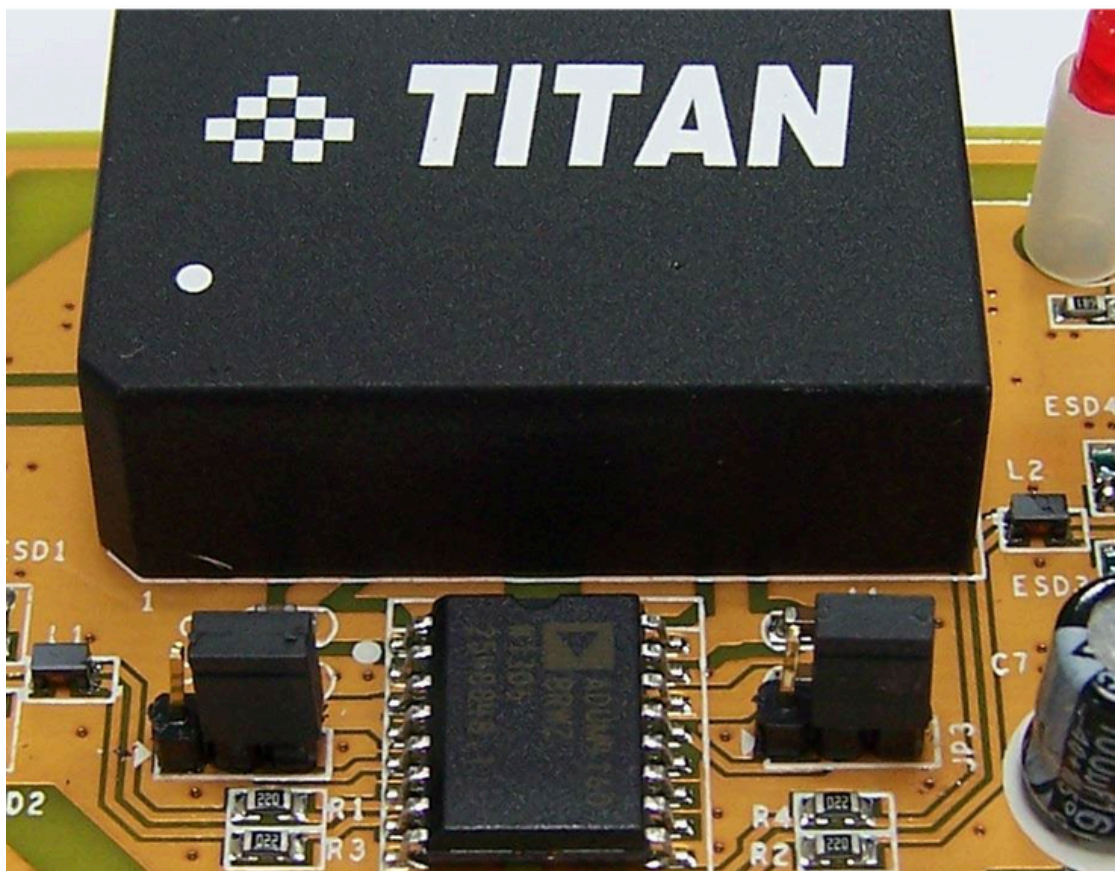
JP2, JP3: pin 2 and pin 3 short for USB1.1 low speed data rate operation
