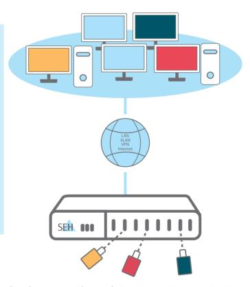
Dongle servers provide an exclusive point-to-point connection via the network. The working principle of USB dongles as copyright protection is not changed, bypassed or eliminated at any time.
