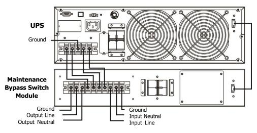
**NOTE:** Make sure that the wires are connected tightly with the terminals.
