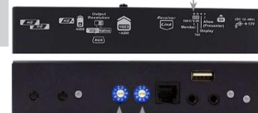
Use the rotary switch to set Row/Column location for the member unit.
