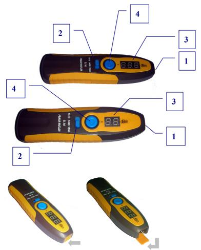
Lift the Dust Cap for access to the connector
