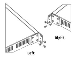
Step 2: Use the supplied M6 screws and cage nuts to securely attach the mounting brackets to the cabinet.
