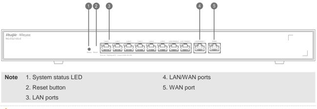
Reset button: Press the button for less than 2 seconds, the system will restart; press for more than 5 seconds until the system status LED blinks, the system will restore the factory settings and restart. After the device restores the factory settings, the default management address is <a href="http://192.168.110.1">http://192.168.110.1</a>.
