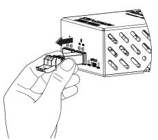
4) Grasp the SFP Module between your thumb and index finger and carefully remove it from the port5) Place the SFP Module on an antistatic mat, or immediately place it in a static shielding bag or container
