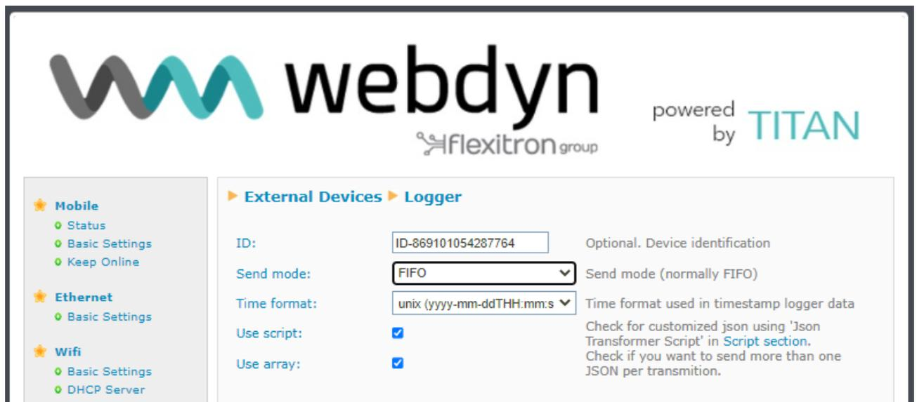
The screenshot shows the webdyn configuration interface. At the top, there is a logo for 'webdyn' with 'flexitron group' underneath and 'powered by TITAN' to the right. On the left, there is a navigation menu with three main categories: 'Mobile' (Status, Basic Settings, Keep Online), 'Ethernet' (Basic Settings), and 'Wifi' (Basic Settings, DHCP Server). The main content area is titled 'External Devices > Logger' and contains the following configuration options:
