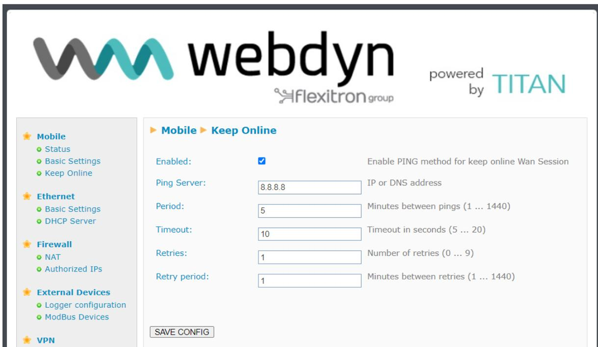
The screenshot shows the webdyn configuration interface. At the top, there is the webdyn logo (a stylized 'w' with a blue wave) and the text 'webdyn powered by TITAN flexitron group'. Below the logo is a navigation menu with categories: Mobile, Ethernet, Firewall, External Devices, and VPN. The 'Mobile' category is selected, and the 'Keep Online' sub-menu is active. The main configuration area is titled 'Mobile > Keep Online' and contains the following settings:
