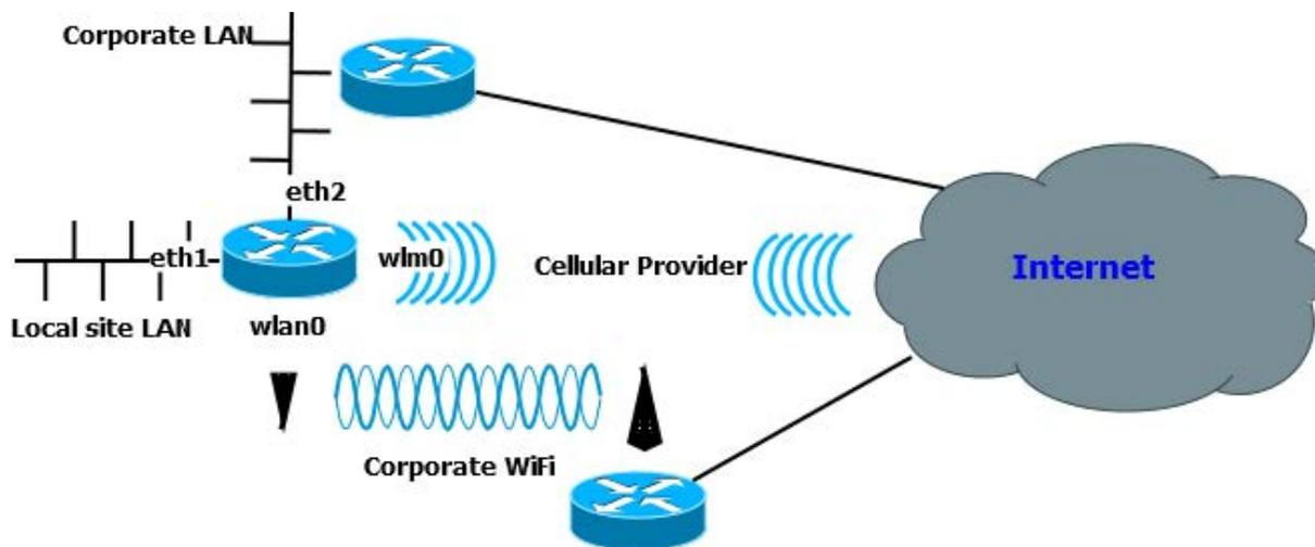
The above diagram shows an example of where a customer wants all his local site LAN traffic on eth1 to by default over his Corporate LAN on eth2, but if that fails, they want all the traffic to go through the Corporate WiFi on wlan0 and if that fails go through the Cellular connection on wlm0 in that order of priority. This means that if both eth2 and wlan0 network connections comes back up it would switch back to the corporate LAN eth2.
