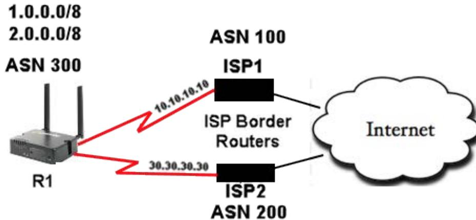
This configuration allows Router (R1) to peer with BGP speakers in other autonomous systems. The **route-map localonly** command allows only the locally generated routes to be advertised to both of the ISPs. This prevents Internet routes from one ISP to the other ISP and prevents the risk that your AS becomes a transit AS for Internet traffic.
