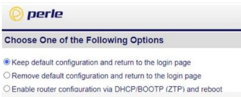
Enabling router configuration via DHCP/BOOTP (ZTP) and reboot, will cause the router to reboot and it will attempt to download either a new version of firmware and/or new configuration from a DHCP/BOOTP server.
