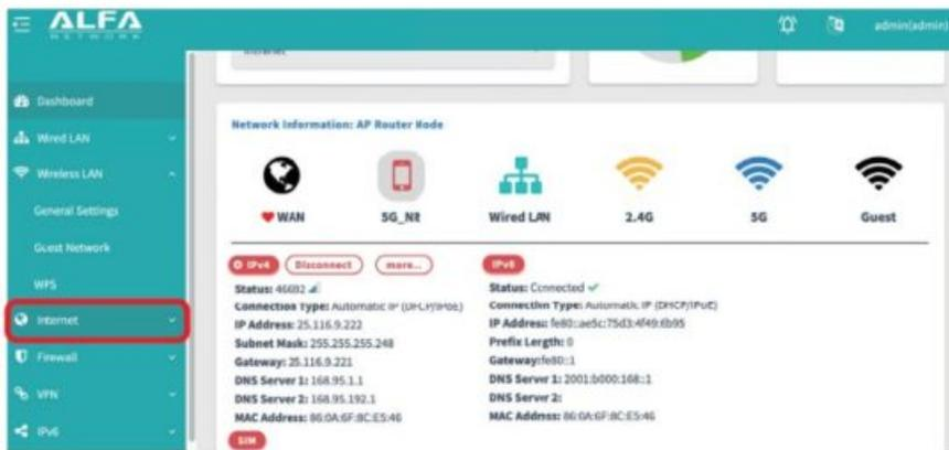
When you insert valid and unlock SIM card from Telkom, the device will auto connect to Internet without setting. If special Telkom SIM card need to set APN, you need to go to Internet item to setup it
