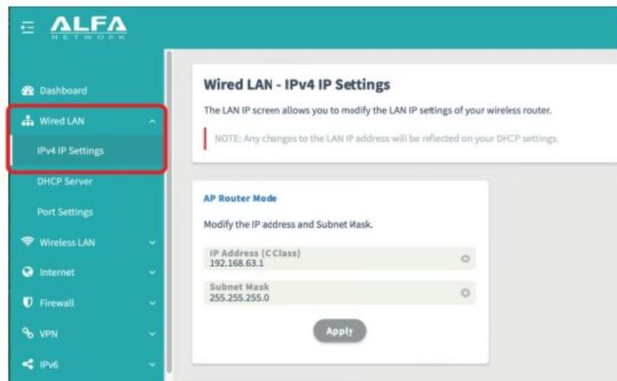
The device default LAN IP address setting is 192.168.63.X, default gateway is 192.168.63.1. If you want to change LAN IP setting, Please go to Wired LAN->AP Router Mode and change the IP Address, when you set up ready, please press Apply button.
