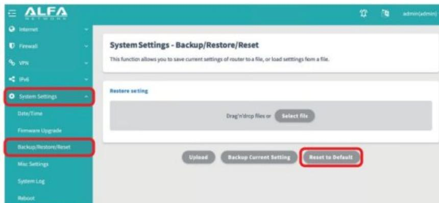
If you want to reset the AX5GRM to factory default setting, please go to System Setting -> Backup/Restore/Reset item. Press Reset Default button. System will process 2 minutes to reset the whole device to default setting.
