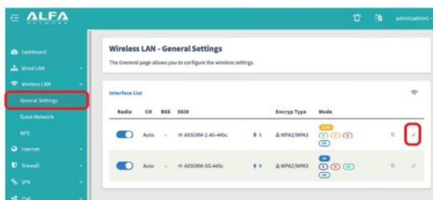
Device with system default WiFi SSID (AX5GRM-2.4G-XXX and AX5SGRM-5G-XXX) and default password (12345678) both on WiFi 11AX 2.4 GHz and 5 GHz. If you want to change your own SSID (WIFI Name) and password, please go to Wireless LAN->General Settings->press edit icon
