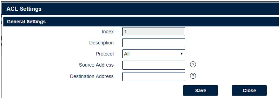
The screenshot shows a dialog box titled **ACL Settings**. It has a **General Settings** section with the following fields: **Index** (text input with value 1), **Description** (text input), **Protocol** (dropdown menu with value All), **Source Address** (text input with a help icon), and **Destination Address** (text input with a help icon). At the bottom right, there are **Save** and **Close** buttons.
